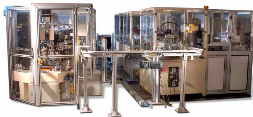
Fig. 1: Development of a fast in-line leak tester based on mass spectrometry as part of a lamp manufacturing line.
