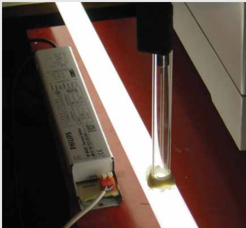
Fig. 3: Monitoring gas phase contaminants in burning fluorescent tubes using mass spectrometry.
