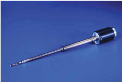
Fig. 1: TEM specimen holder for resistance versus temperature experiments.
