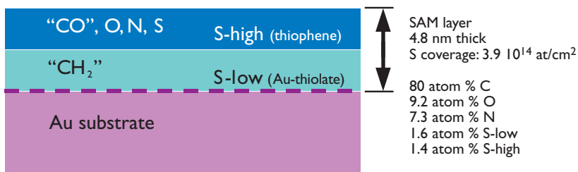
Fig. 7: Multilayer model of BAT on gold (see figure 5). This SAM layer can be seen as two organic layers on top of the gold substrate: a lower layer containing the -(CH_2)_x- part of the molecules and a top layer containing predominantly CO groups and N, O and S of the thiophene group. The S of the thiol group is present at the gold surface only. One single measurement results in the 'raw' concentration. A subsequent model calculation provides the real layer composition, as shown next to the figure.
