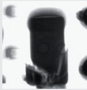
Optical photography image and X-ray images of a Printed Circuit Board (PCB). Inspection shows the malfunctioning component: the crack in the capacitor is clearly visible in the X-ray images.
